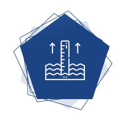
Maintain your pool's water level near to the skimmer's centre point at all times. By allowing air enter the system, a lower level can harm the pump and filter. The effectiveness of the skimmer decreases as the water rises.
